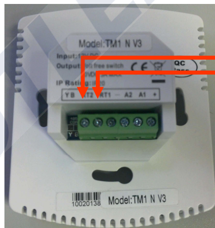
Rear view of timer showing the 2 unused wires
