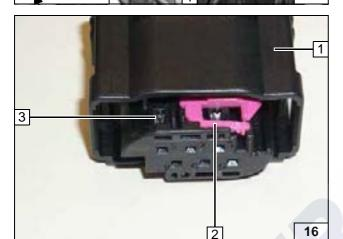
Disconnect 6-pin connector X1 1 from the heater. Unlock secondary locking device 2 of the 6-pin connector (move to the right).
