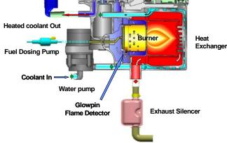
**Operation**– Once activated, the Webasto Thermo Top C heater will use the vehicle's own fuel in a combustion process to heat the coolant via a heat exchanger. The heated coolant is then circulated round the heating circuit passing through the fresh water plate heat exchanger & blower heaters by an integrated water pump. The Webasto unit is self regulating & operates in a similar way to a domestic central heating system.
