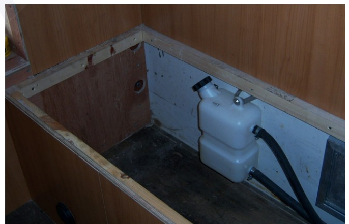
Tank can be mounted vertically or horizontally with left or right fill
