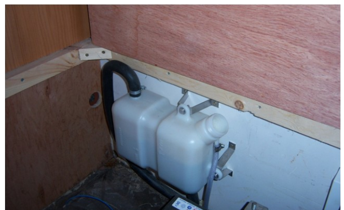
Tank can be mounted vertically or horizontally with left or right fill
