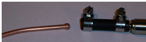
Flared end of copper pipe
