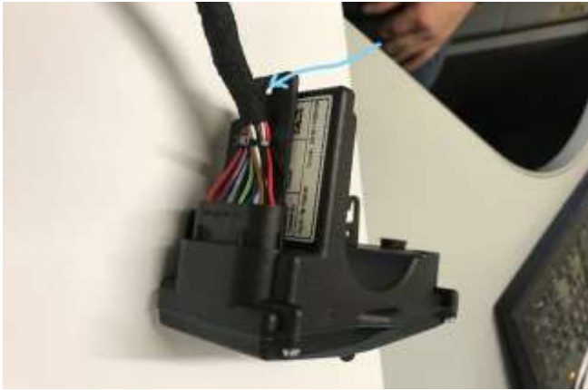
see left, showing locating cut out in plastic plug connector
