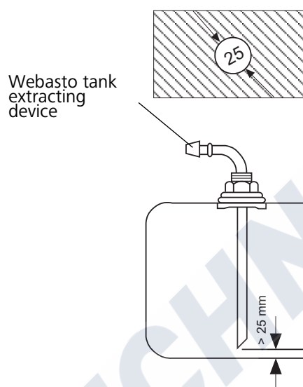
Fig. 804 Webasto tank extracting device (metal fuel tank)
