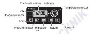
The combination timer allows the heater start time to be selected for
