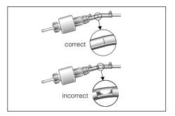
When installing a T-piece, always keep to the mounting positions shown in the drawing.
