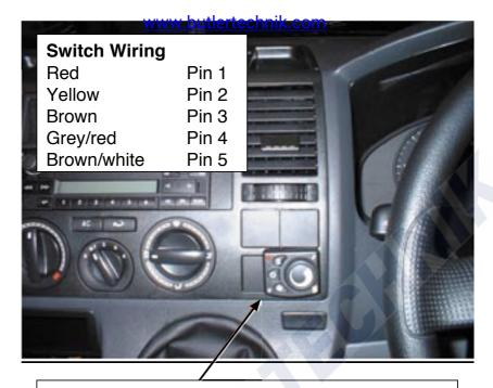
Switch mounted on dashboard onto VW blanks.
