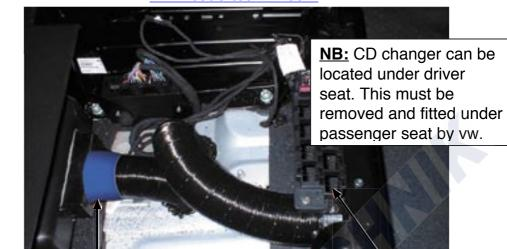
Blue silicone adapter to connect hot air outlet ducting to outlet.
