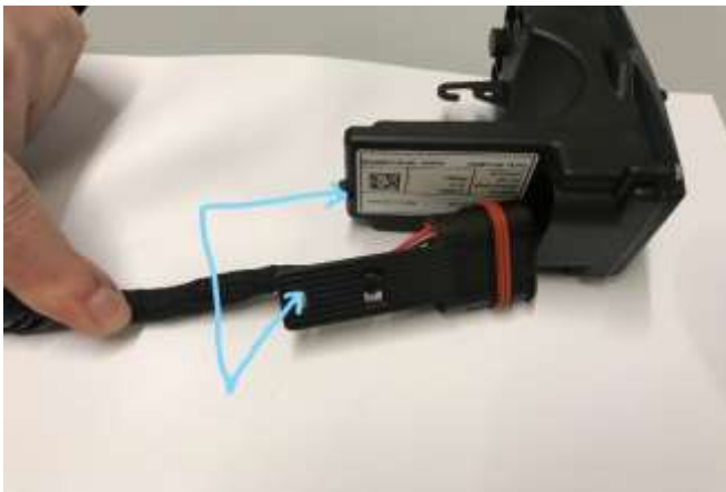
see left, showing tab on ECU that MUST be located within the cut-out on the electrical plug connector
